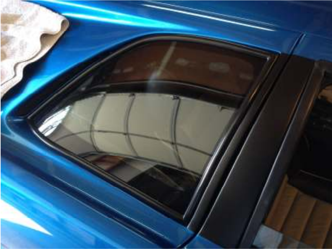
Quarter Glass installed
