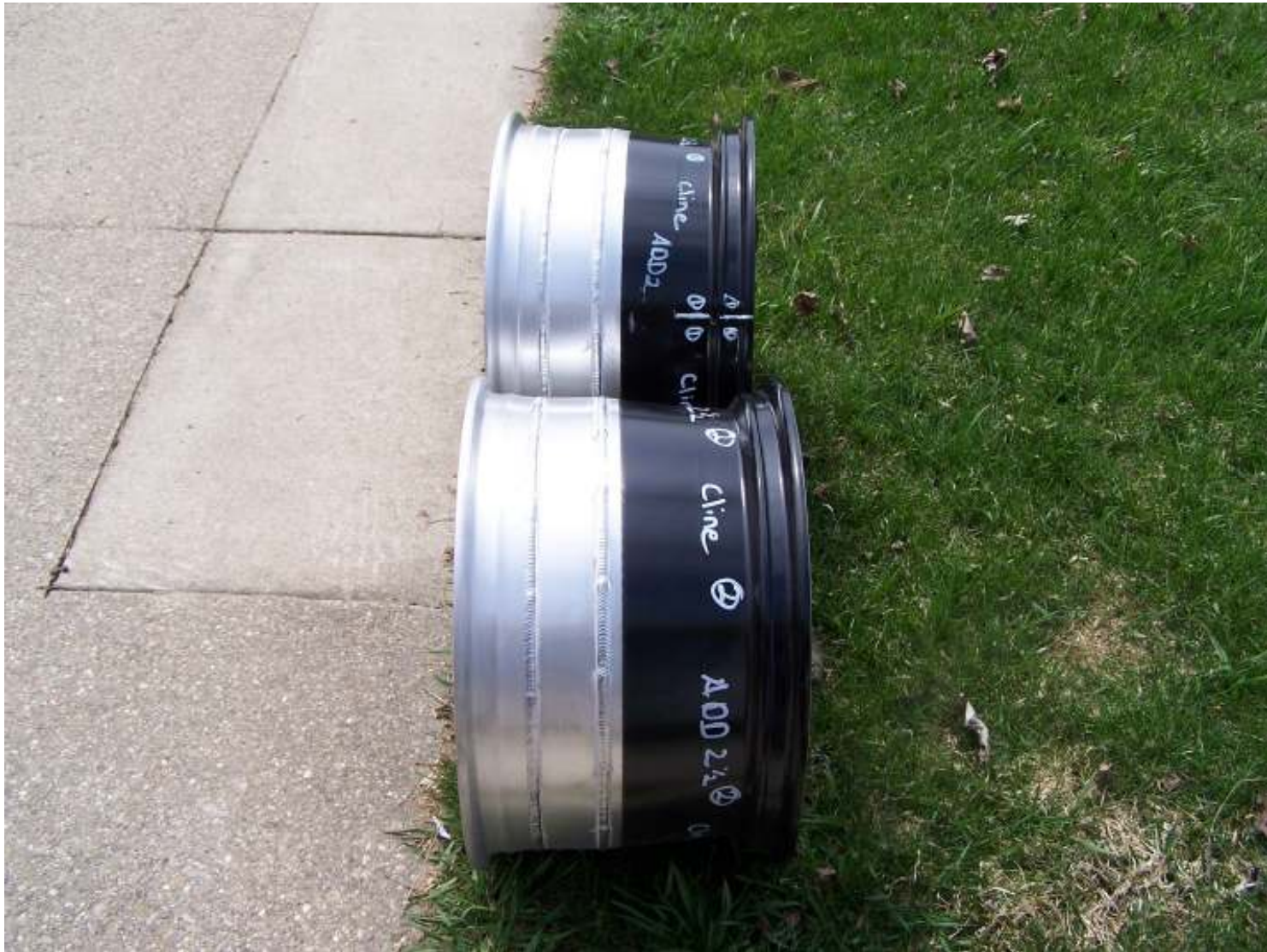
Pic #110 I sent my rear wheels to Weldcraft in Livonia, MI to have them widened 2.5"
