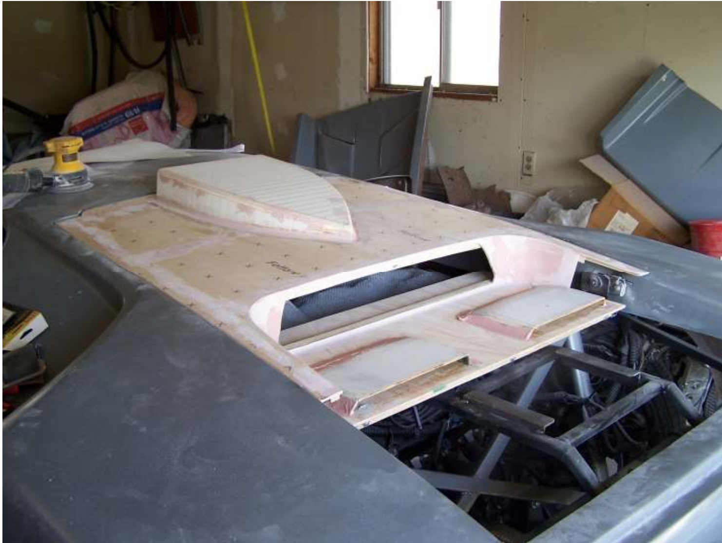
Pic #107 A little bondo to smooth out edges.
