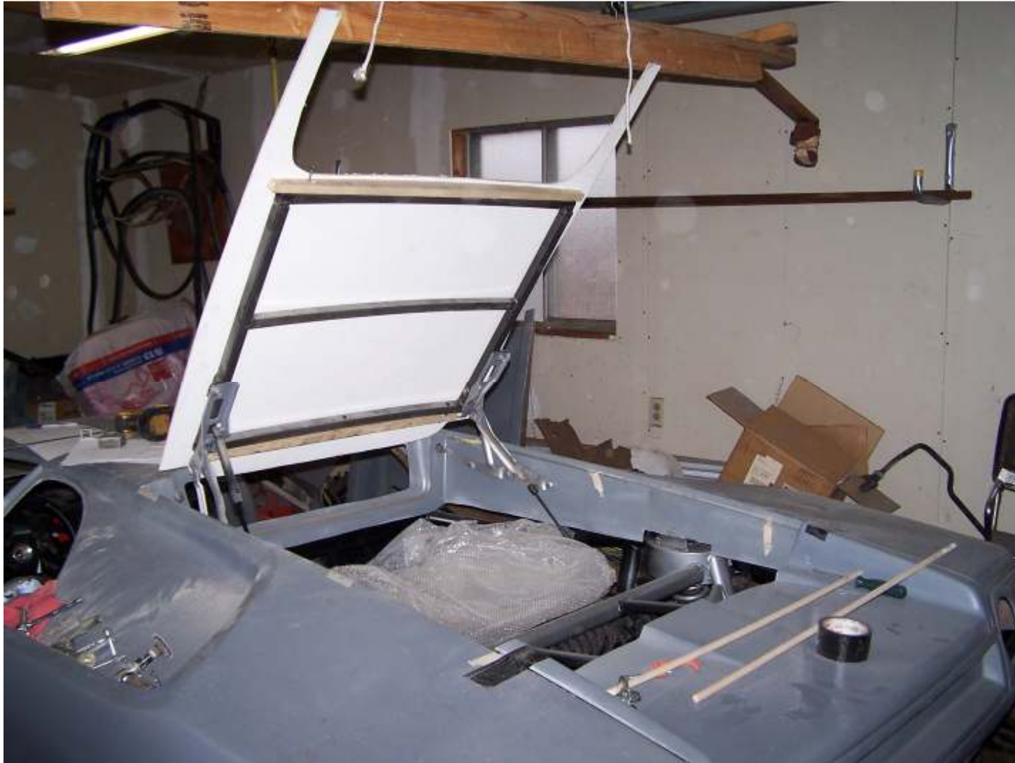
Pic #102 Plywood attached to partial cover.
