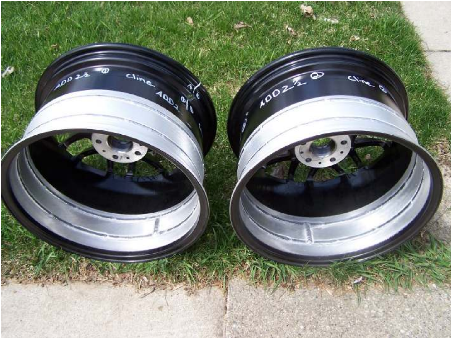
Pic # 111 I sent my rear wheels to Weldcraft in Livonia, MI to have them widened 2.5"
