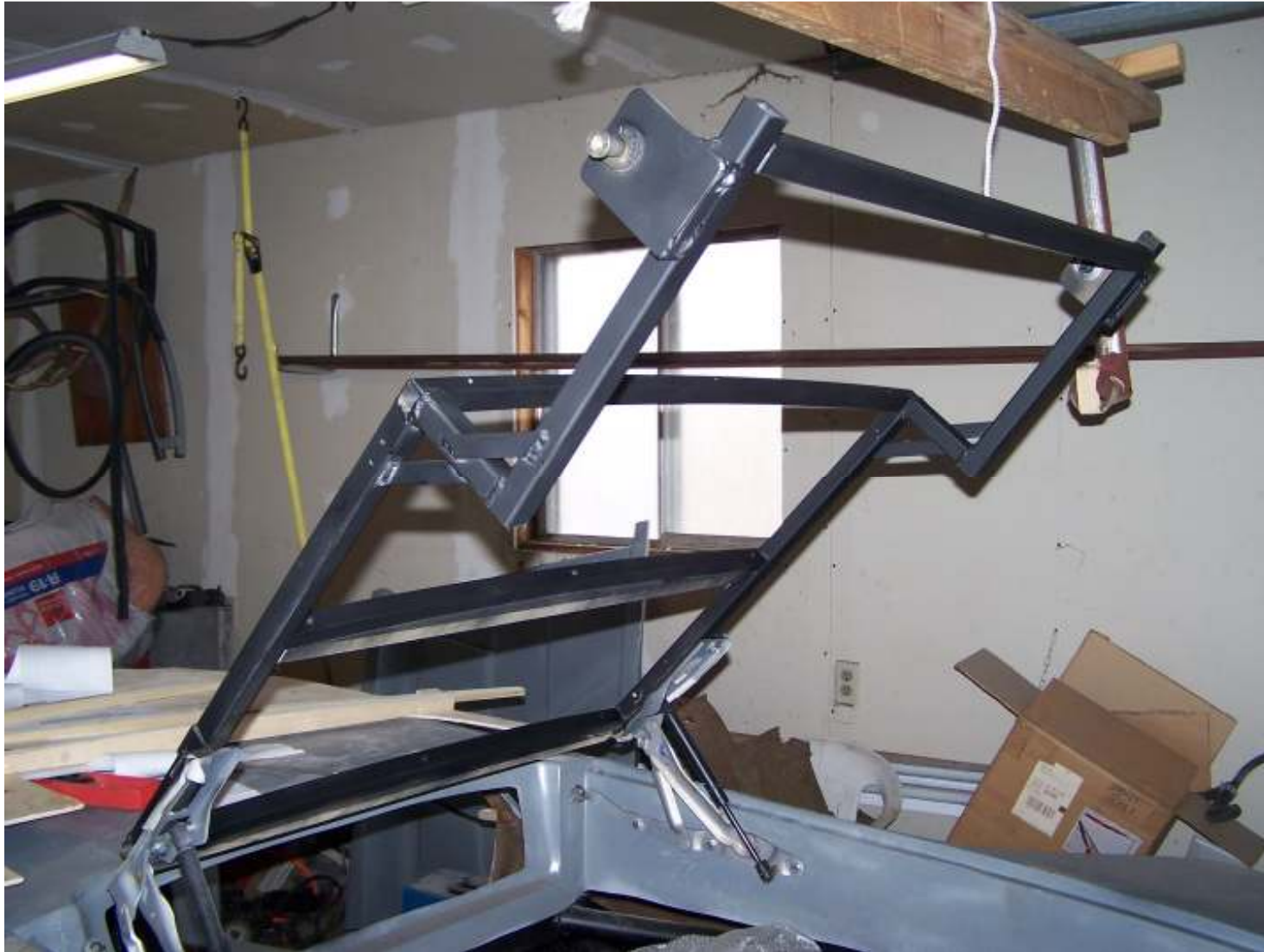
Pic #104 Complete framework for cover with Bearclaw strikers.
